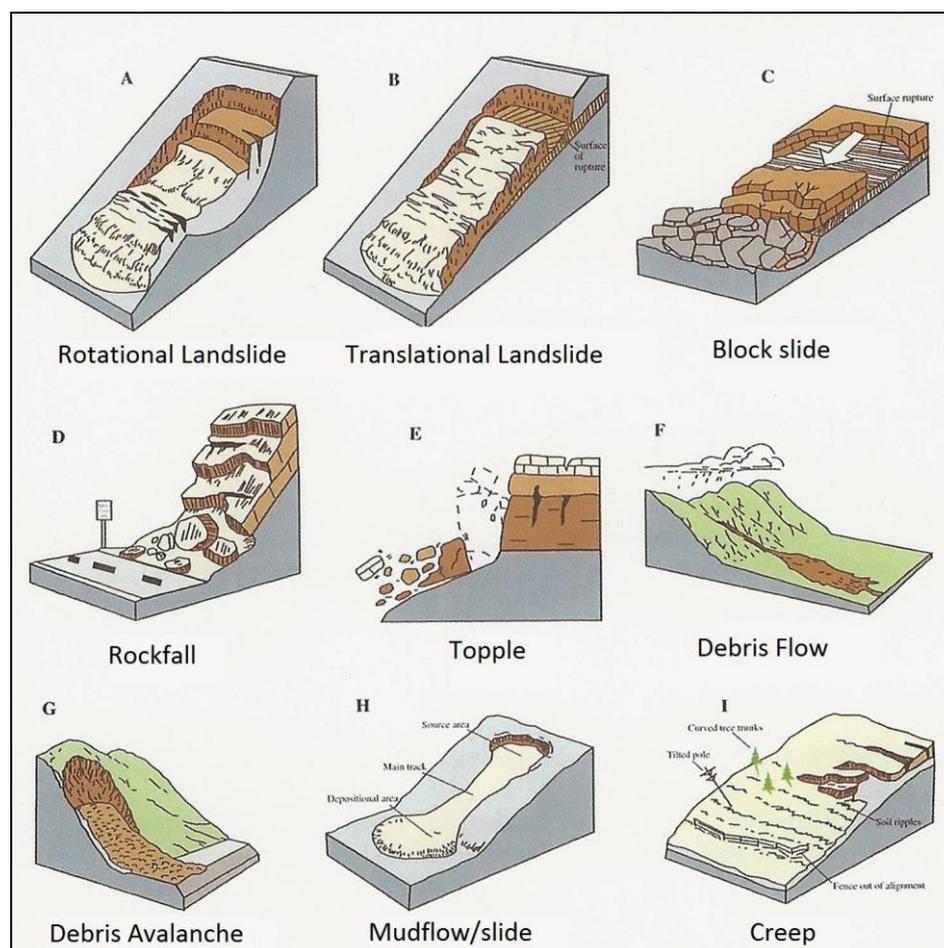
Figure 4: Examples of landslide mechanisms and mass wasting processes occurring in Great Britain (from Moore & McInnes, 2011).
