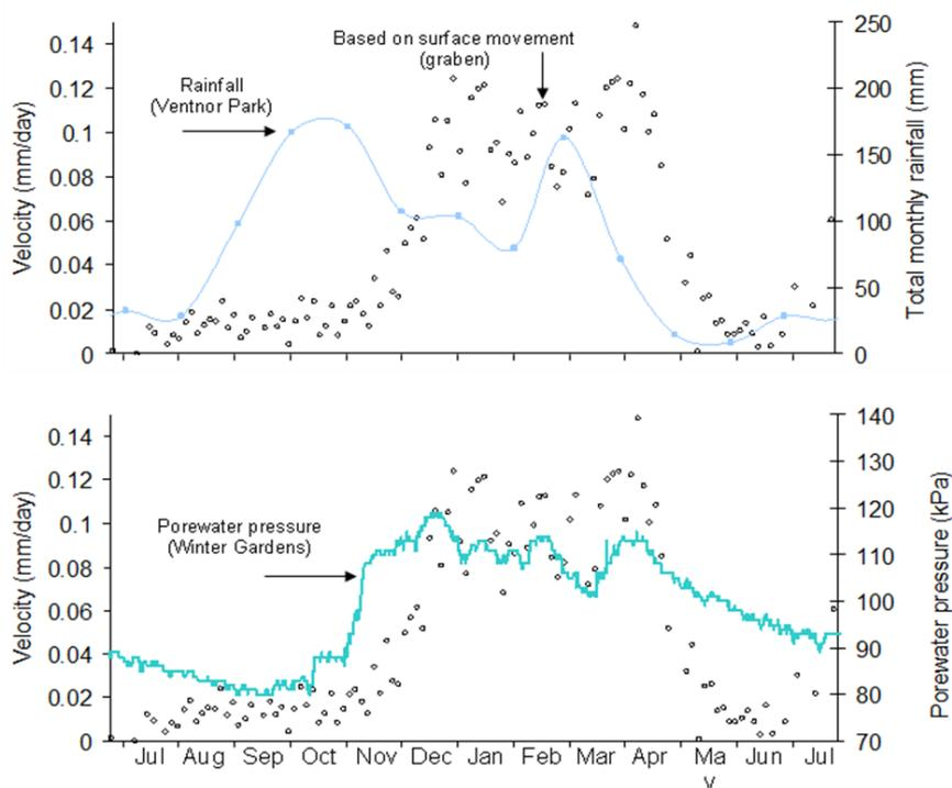
Figure 5: Relationship between rainfall, pore-water pressure and ground movement at Ventnor, Isle of Wight (Moore et al, 2010).
